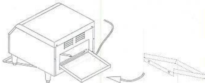
Rear slag palte installation diagram
