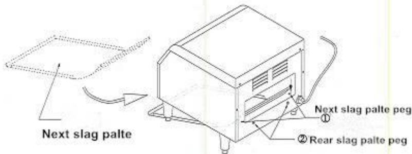
Next slag palte installation diagram
